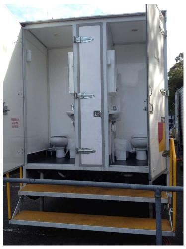
The truck can be powered off mains supply, or it runs off its own 7kva Honda generator. All stairs have hand rails for safety. This combo has a water tank that can hold half a tonne. It has two separate waste tanks for the toilets, and grey water tank for the sinks.
